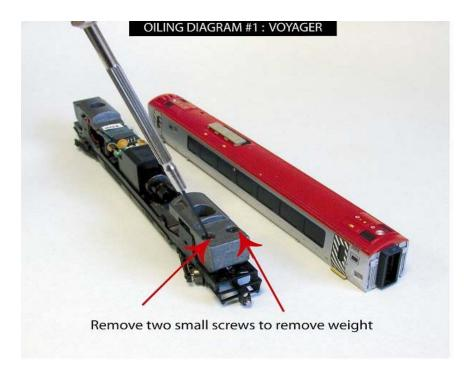
Once the weight is removed you can see the exposed top gear in the bogie tower. Both this and the silver pin need to be lubricated to aid dispersion of the transit grease that the model comes with, or indeed just to lubricate the harder to get at areas.
