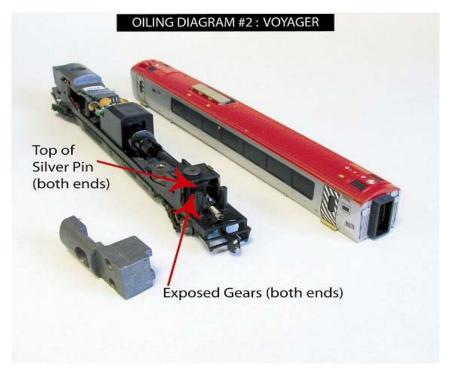
Once you have lubricated this end of the motorised unit, replace the weight and screw down firmly. then do exactly the same with the other end.
